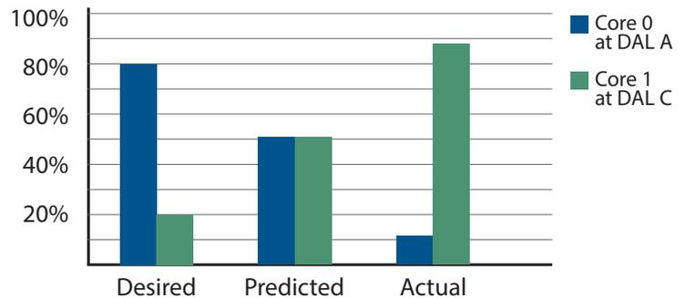
**Figure 2:** Example memory access bandwidth for DAL A and DAL C applications on different processors trying to access DRAM simultaneously.
